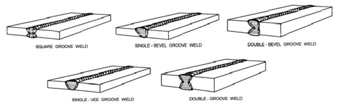
Groove welds may be joined with <u>one or more</u> <u>weld beads</u>, depending on the thickness of the metal. If two or more beads are deposited in the groove, the weld is made with <u>multiple-pass</u> <u>layers</u>, as shown in the figure. As a rule, a multiple-pass layer is made with stringer beads in manual operations.
