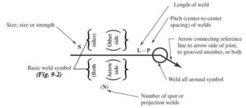
• The table shows the *Basic weld symbol* for the different types of welds.
