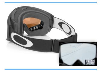
US eyewear brand **Oakley** has already demonstrated a practical application for wearable 'KNOW' devices. In October 2012, the brand launched its Airwaye Ski Goggles, which feature integrated Bluetooth and GPS. The goggles deliver real-time performance analytics and navigational information in front of the skier's eyes, with information delivered on a prism technology display to avoid optical re-focusing. The goggles retail at USD 599.
