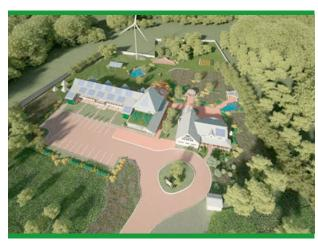
Scheduled to open in Q3 2013, **The Green Leaf Inn** in Delavan, Wisconsin is a net-zero energy hotel that will generate more electricity than it consumes. The boutique hotel includes an on-site aerobic wastewater treatment system, a wind turbine, multiple solar panels and a rainwater collection program. Rooms are equipped with en-suite bathrooms and hot tubs, while QR codes enable guests to discover more about the energy initiatives throughout the hotel.
